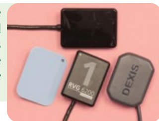
Figure 1: Large sensors (top) can be difficult to position. Options include phosphor plates and smaller sensors.
